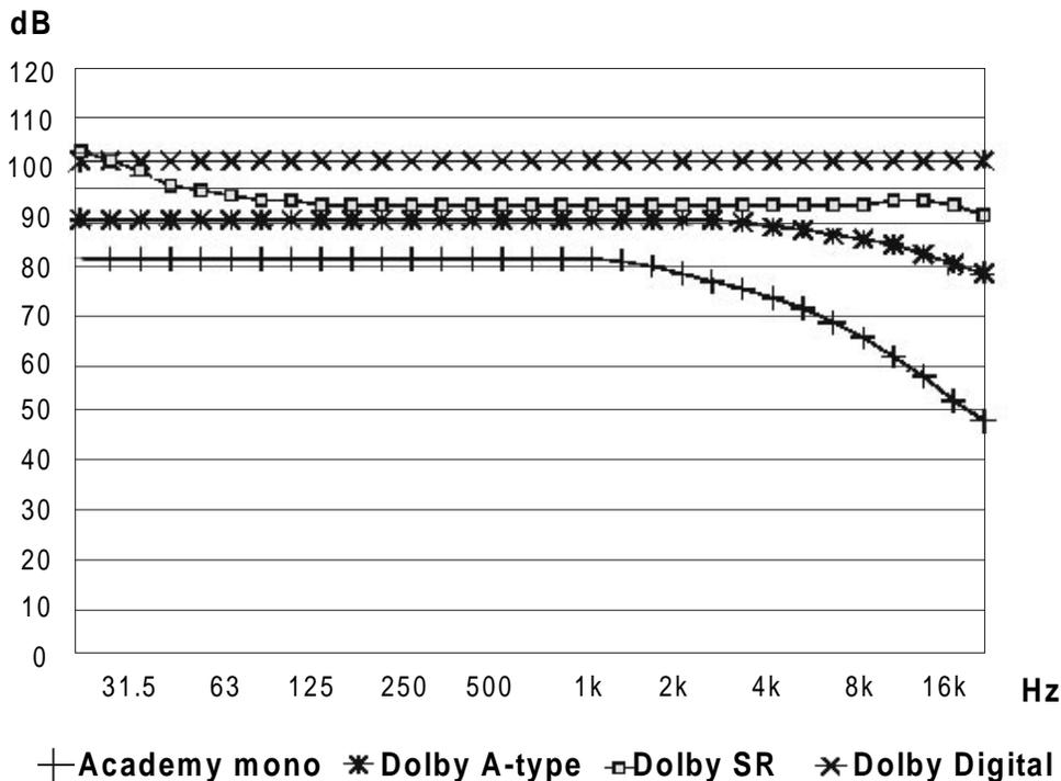
**Figure 1** Peak levels of photographic soundtrack formats
